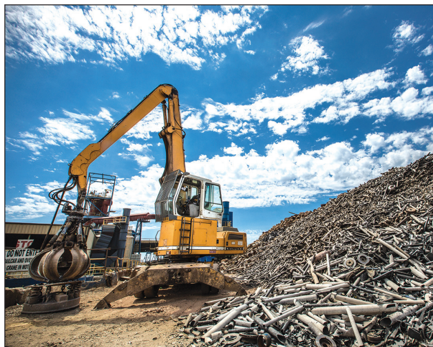
AB&I Foundry's cast iron soil pipe and fittings are made from 95 percent post-consumer scrap metal, which reduces the demand on landfills.
