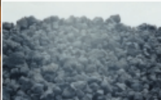
Coke fuels the furnaces that melt the iron in the foundry.
