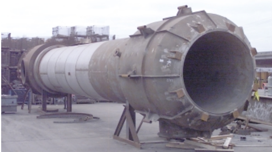
AB&I's new recuperator awaits installation at the Oakland headquarters.
