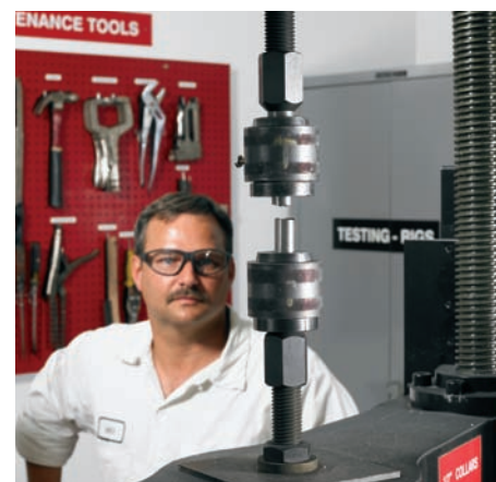
CISPI requires a tensile strength test, as shown, to be conducted every four hours to ensure iron quality.
